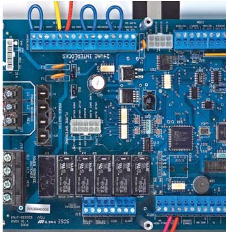
variety of set-up configurations – as a stand-alone boiler, a boiler in a Master/Member network using HeatNet protocol, or as a member in a system for up to 16 boilers. HeatNet provides a higher
